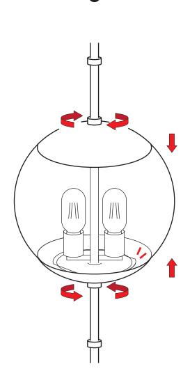
Rotate glass to slide it back. Globe shoud rest on plate.
