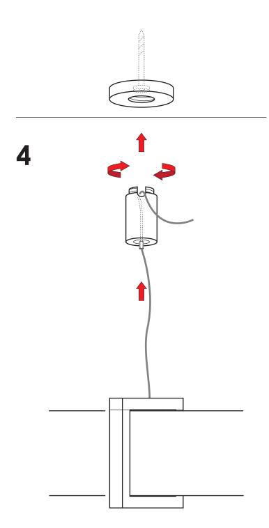
Thread wire through lock. Connect lock to ceiling.
