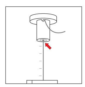
Lower lamp by pushing in small bottom cylinder.
