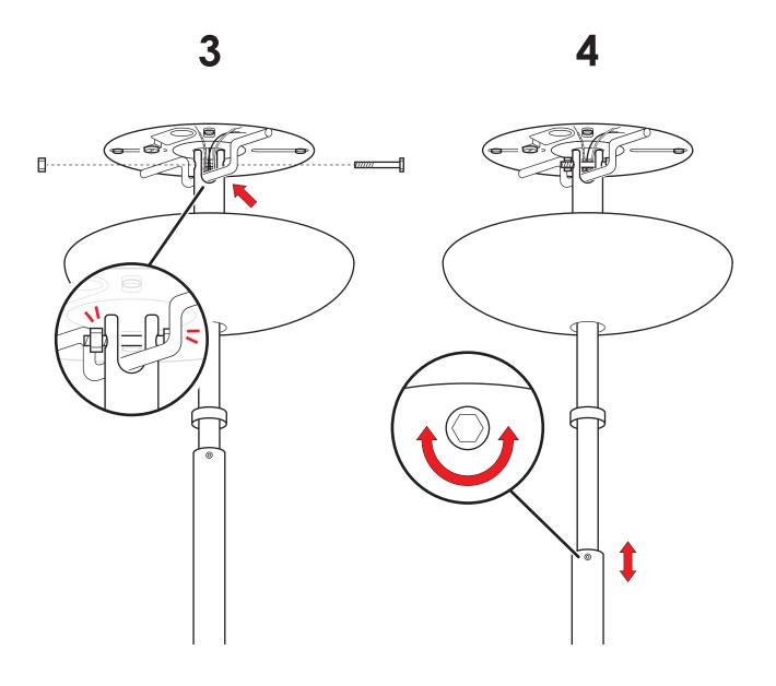
Adjust height of telescope.
