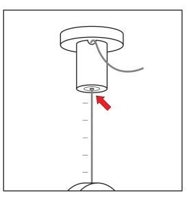
Lower lamp by pushing in small bottom cylinder.
