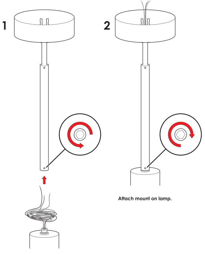
Thread wires from lamp through ceiling mount.
