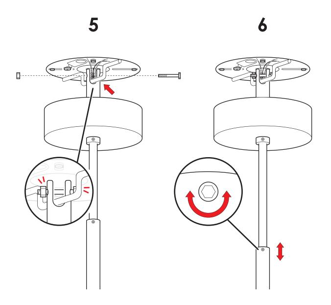
Adjust height of telescope.
