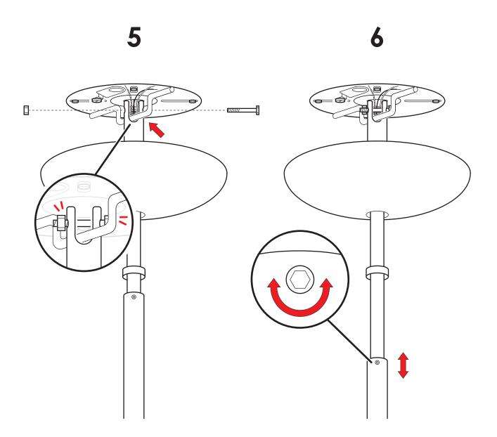
Adjust height of telescope.
