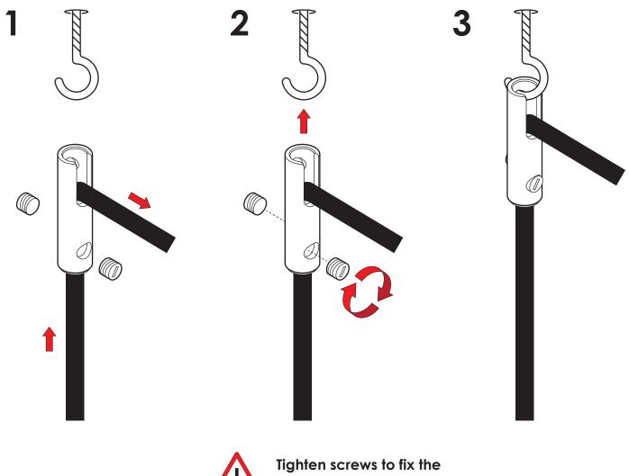
Tighten screws to fix the cord in the bracket.
