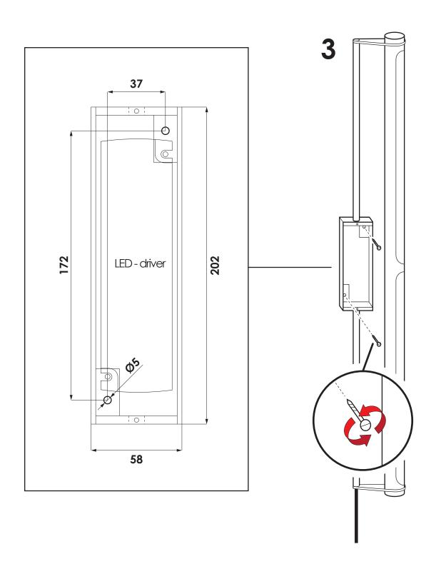
Mount on wall using 2 screws (not included).
